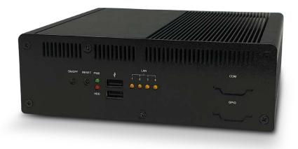
Part of the EkkoSense Critical Things<sup>®</sup> family of monitoring technology, EkkoLink CM operates as a data aggregator – receiving data from EkkoHub wireless data receivers and securely forwarding it over a wired or cellular Internet connection to EkkoSoft<sup>®</sup> Critical software in the cloud
